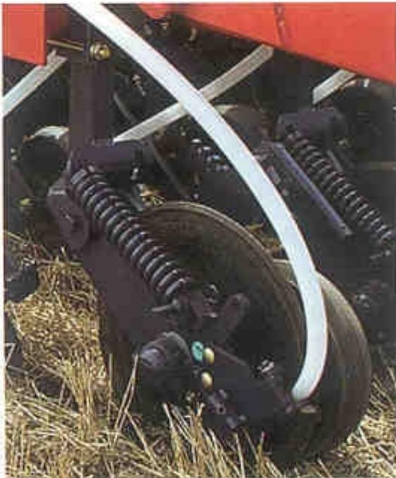
Fig. 8: Disc edge bevel position influences smearing risks with angled coulters (eg. *Morris* fertiliser opener design shown)
