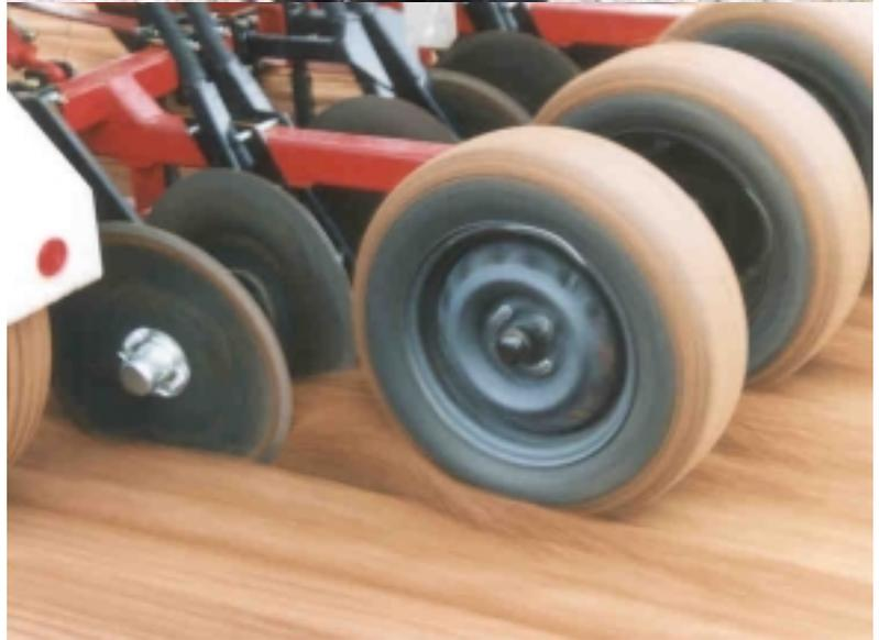
Fig. 9: NSW disc seeder development featuring paired undercut discs working in opposition and spaced apart to loosen a narrow band of soil. At speed, a soil wave is formed under which seeds are delivered followed by a wheel squashing action achieving furrow closure. Principles of the paired disc loosening process were investigated in the UK in the mid 1980s which demonstrated higher energy efficiency under optimum settings (eg. *Wyalong Rene* speed drill design shown)
