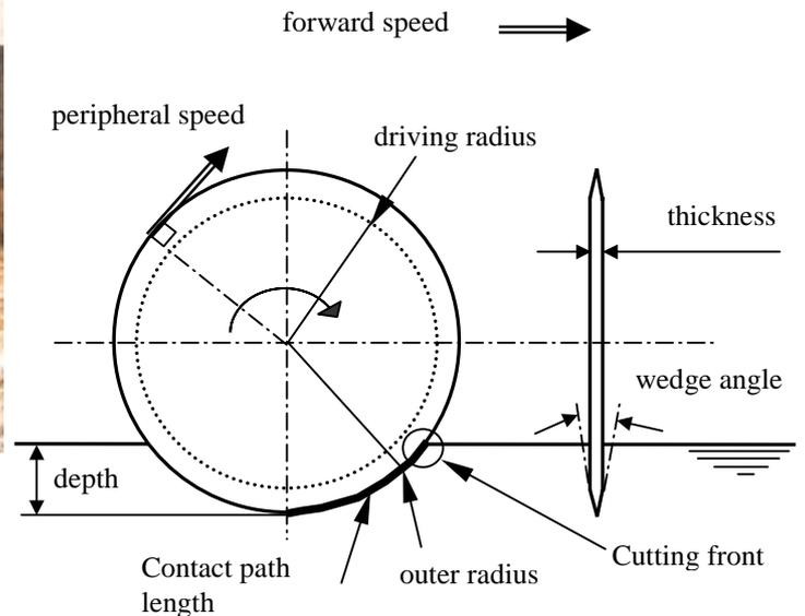
**Fig. 5: Basic disc coulters geometry**
