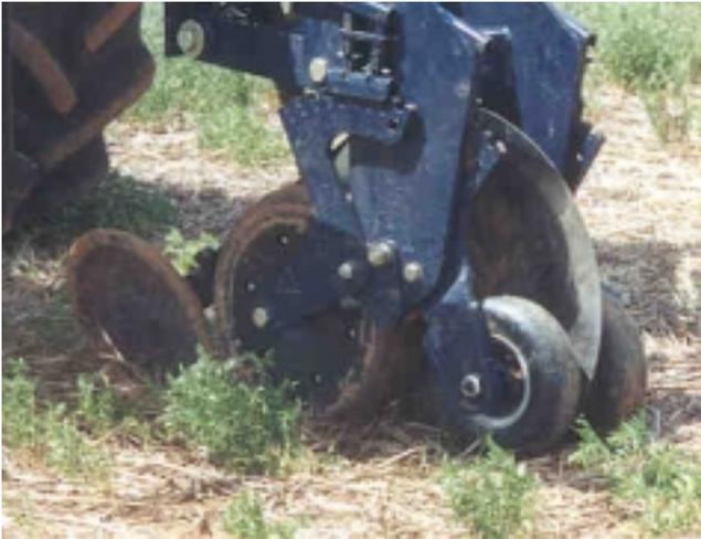
Fig. 7: Pincher wheels can help cutting through residue provided enough extra pressure is available beyond that required for disc penetration, without inducing wheel sinkage in soft soils (eg. Morris *Never Pin* design shown)
