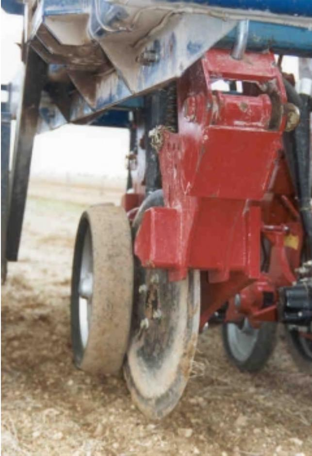
**Fig. 3: Angled disc openers develop side forces and are associated with a side wheel, which may have some or all of the following functions: soil throw control, disc cleaning, depth gauge and furrow closing. Its position and orientation relative to the disc influences disc cleaning ability and can affect draft requirements. (eg. Milne industries *Day-Break* design shown)**
