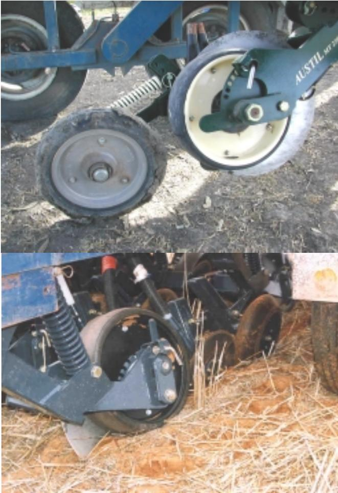
**Fig. 4: Undercut disc openers offer superior penetration ability in hard ground with greater associated soil disturbance (eg. Flexi-Coil Barton – top- and Austil MT2500 – bottom - dual banding designs shown)**
