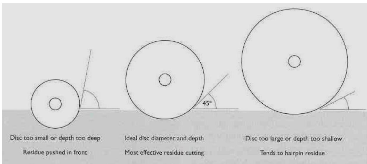
Fig. 6: There is an optimum working depth for residue cutting with any given disc diameter
