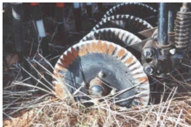
Fig. 2: Swivel type, fertiliser banding and parallelogram mounted disc coulters – the ripples result in improved driving ability compared to smooth discs (eg. Yetter design shown)
