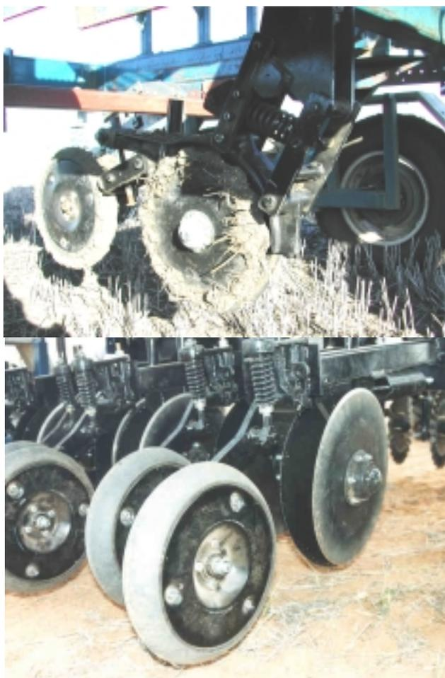
Fig. 1: V paired disc designs typically offer very accurate seed placement in non-sticky conditions. With one pass zero-till systems, they best operate in a triple coulters layout (eg. behind an additional deep working coulters disc offering deep soil disturbance, residue cutting and fertiliser banding benefits) – *Agrowdrill* – top - and *K-Hart* designs shown
